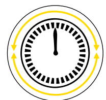
Rotatable dial, for zero setting of the scale
